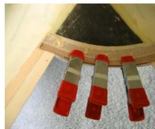
Next I had to reinforce the inside of the fuselage where the hatch was about to be cut out. I did this by gluing in material all the way around.
