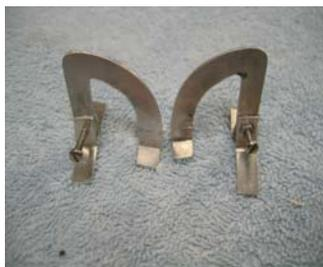
First, I made some hinges that I thought would allow the window hatch to open out and up. Essentially, I made a mock-up out of cardboard and then when I was satisfied with the size, I fabricated them out of aluminium.
