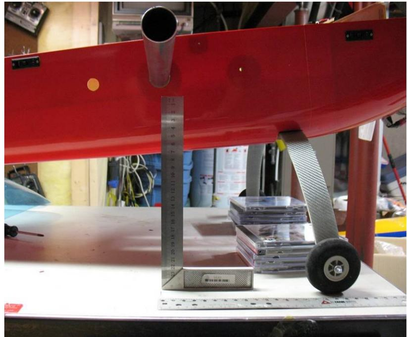
Now, here's the magic of this method. Usually you know where you want the CG to be. You can reverse the equation above, so that if you know where the CG should be, you can figure out what the weight of the tail wheel should be:
