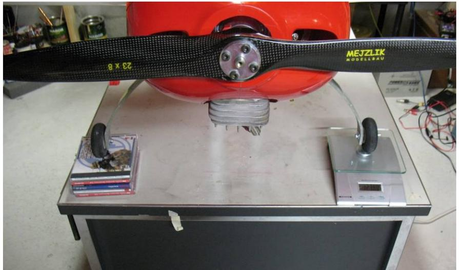
5. Swap the scale and CD cases, and record the weight measured by the scale under the other main gear. On my Katana, the weight at this wheel was 125.6oz.
